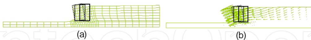
Figure 9. Computed post-earthquake (a) deformed shape, (b) nodal displacement vectors for the quay wal after the seismic loading
