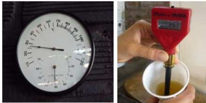
Figure 4. Thermohygrometer and pH-meter
