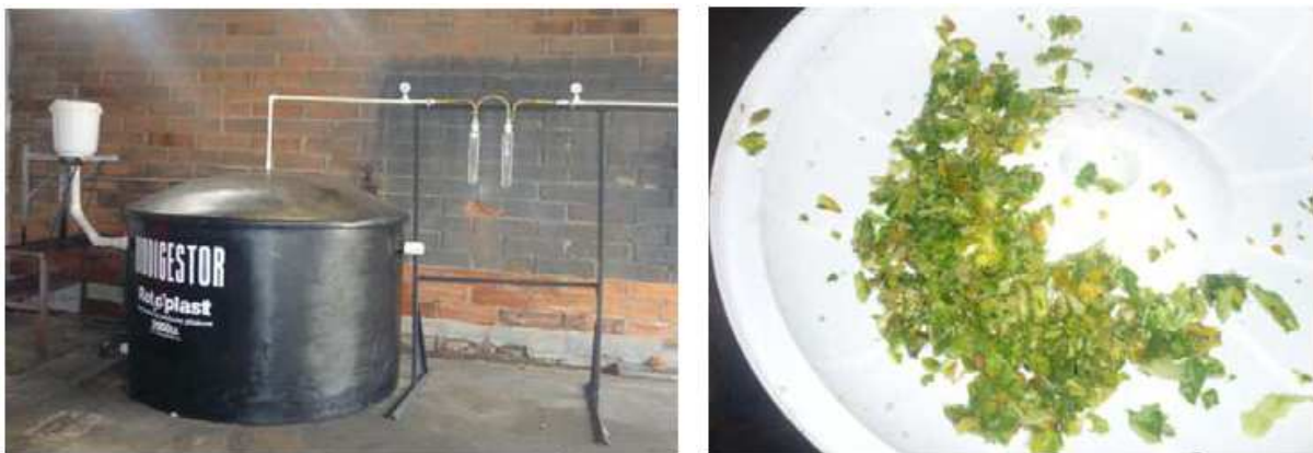
Figure 8. Bioreactor used by the first stage and wastes triturated
