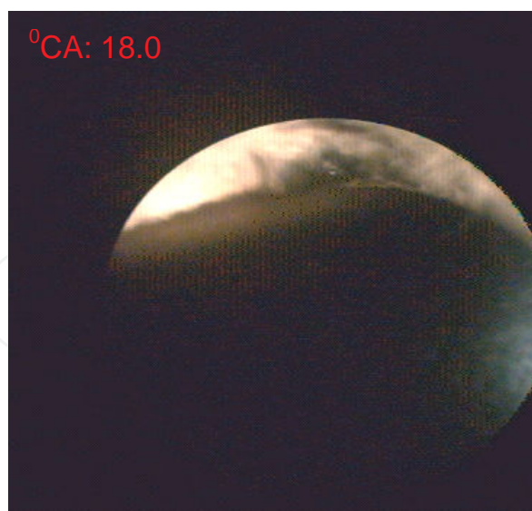
Figure 27. Moment of ignition took place for 10 deg CA before TDC. The photograph present the initial phase of flame development for 18 deg CA after TDC. High whirling occurring in the combustion chamber is clearly visible.
