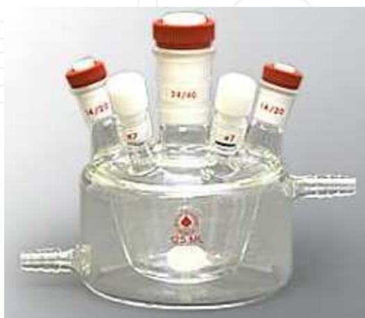
Figure 1. Electrochemical cell used for cyclic voltammetry experiments.
