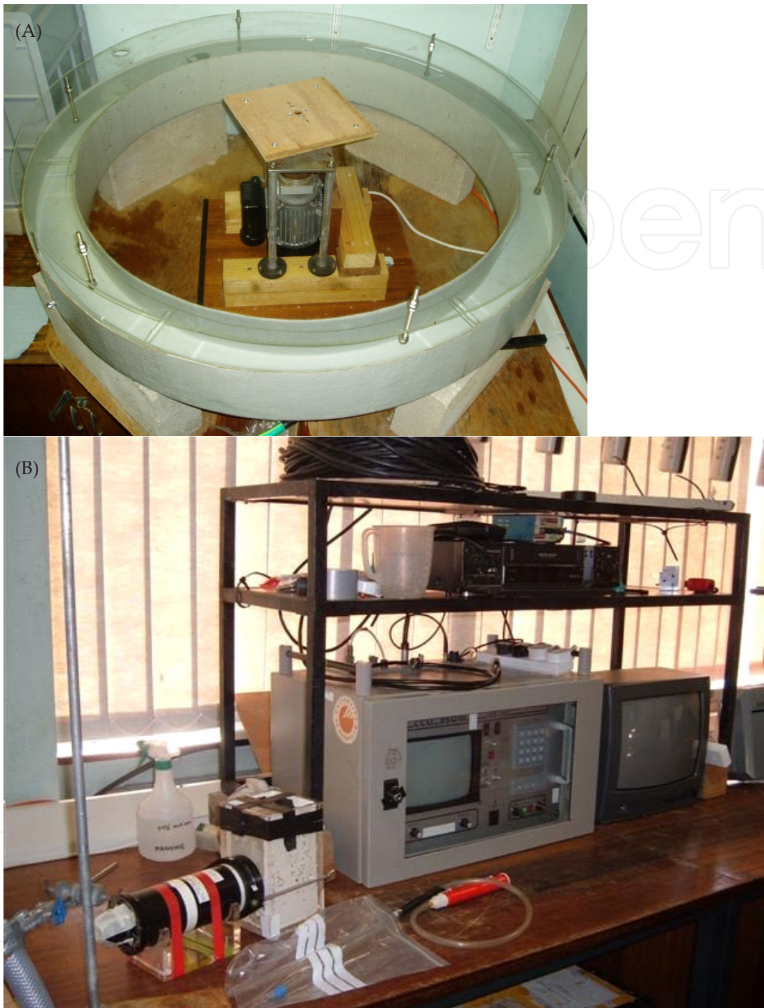
Figure 3. The mini-annular flume (A) and the LabSFLOC instrument set-up (B).
