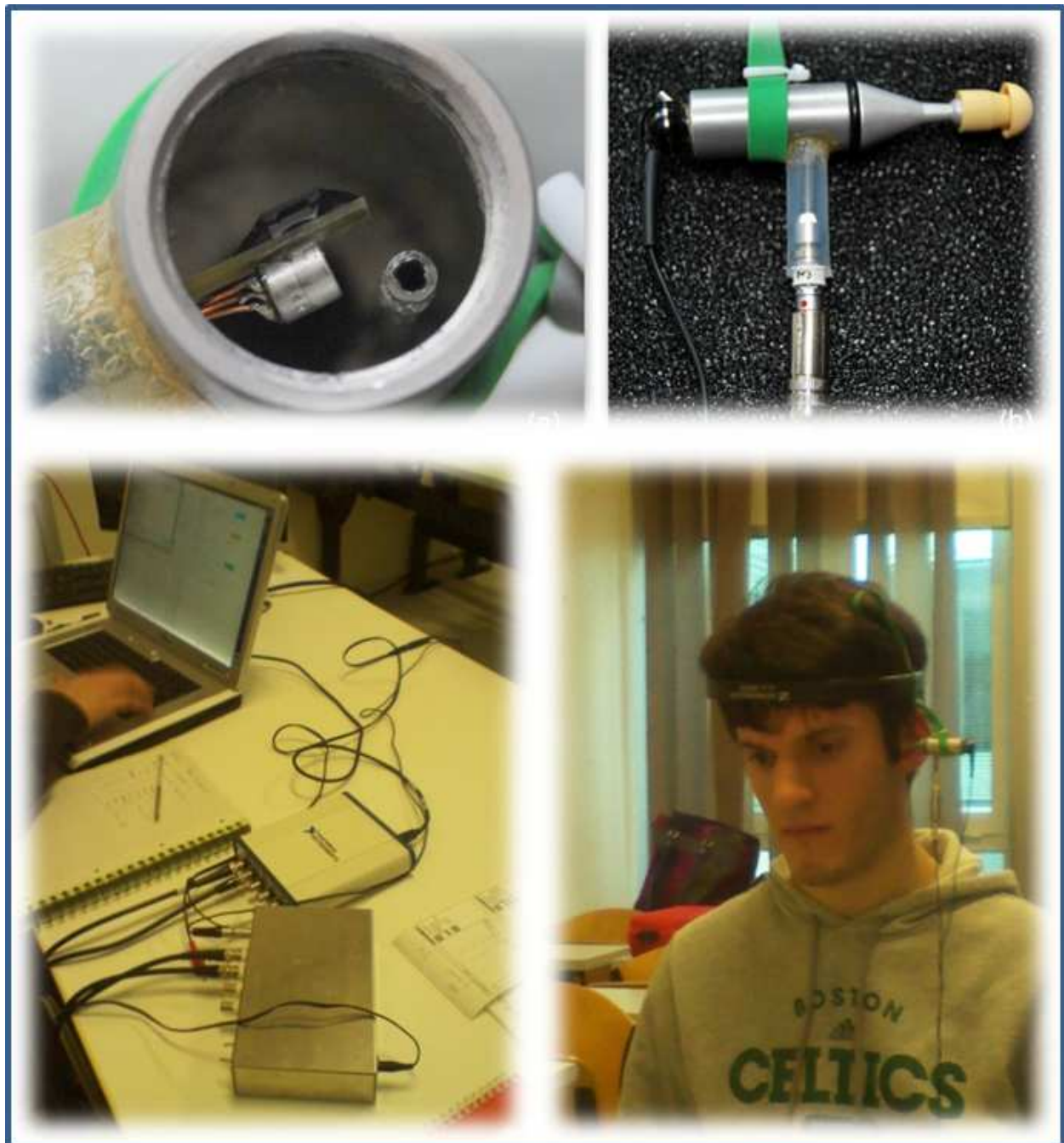
Figure 5. A p-v tympanometer is designed as a laptop based dual channel analyzer (lower left) able to record both the Impulse Responses (IRs) of pressure and velocity signals captured with the p-v tympanometric probe shown in the upper part of the figure. Once the p-v IRs of the ear canal have been measured in atmospheric pressure condition (lower right), the system calculates the external/middle ear specific immittance and displays its magnitude in dB relative to the frequency dependent baseline Y_0 obtained by plugging up the probe.
