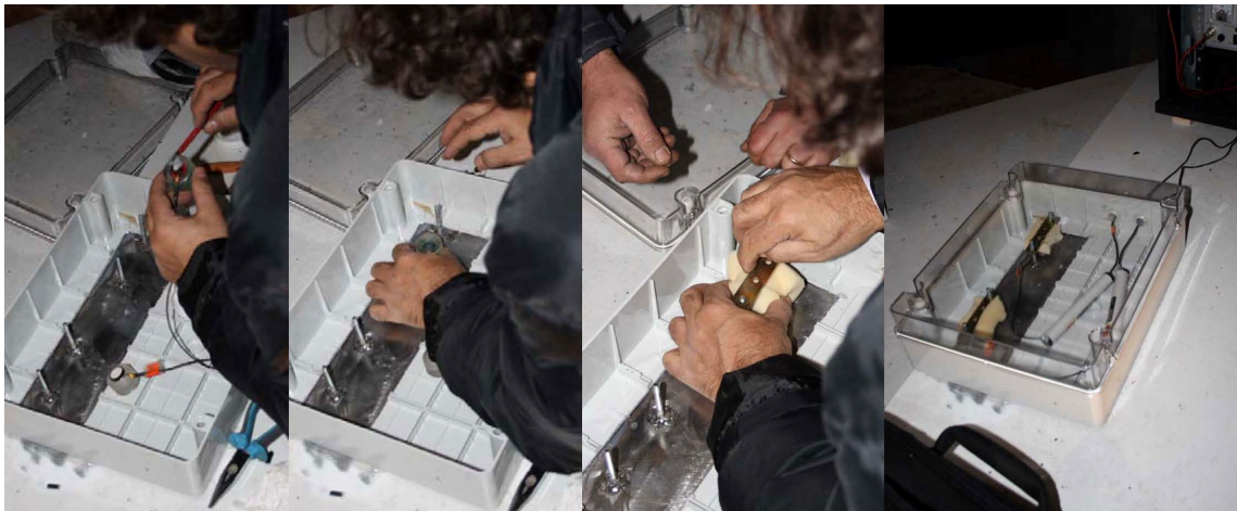
Figure 5. The AE recording apparatus while it is implemented (upper figure), and details of the AE detector (lower figure), where every AE transducer is located inside a transparent plastic cylinder (left figure), and the two preamplifiers are the small white cylinders (right figure).
