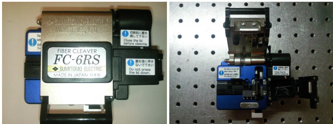
Figure 84 – An image of the cleaver that was used to cleave the fiber tips.
