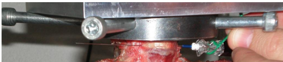
Figure 48 – Ventral view of the spinal motion segment. A needle was used to perforate the intervertebral disc from side to side and guide the sensor into the center of the disc.
