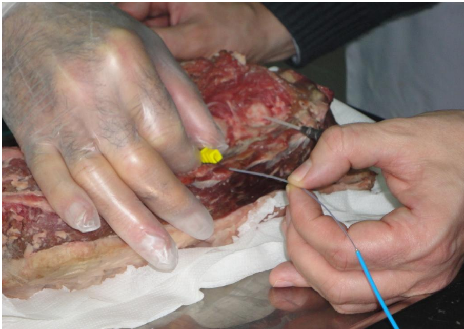
Figure 64 – Insertion of the Samba sensor into the needle lumen.
