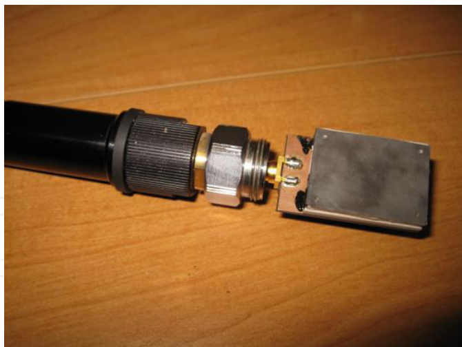
Figure 16. Model of antenna during VSWR measurements.
