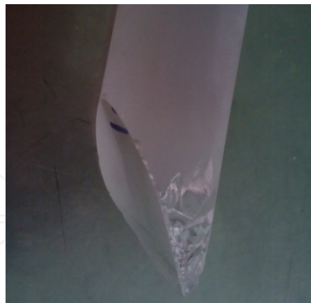
Figure 27. Cracking in the sapphire rod with stress.
