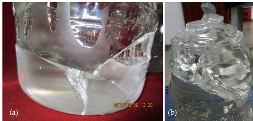
Figure 26. Cracking in large size sapphire crystals: (a) stress cracking, (b) polycrystalline cracking.
