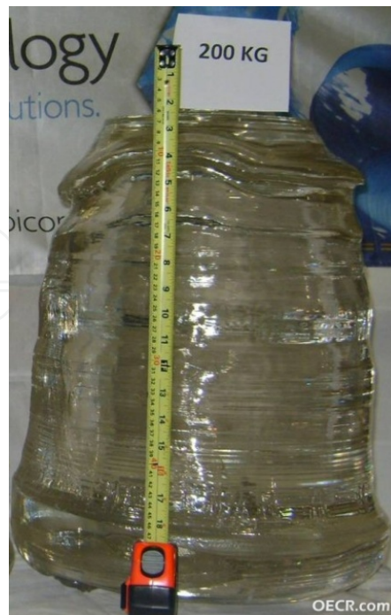
Figure 9. Sapphire boule grown by Rubicon Technology Inc.[17].
