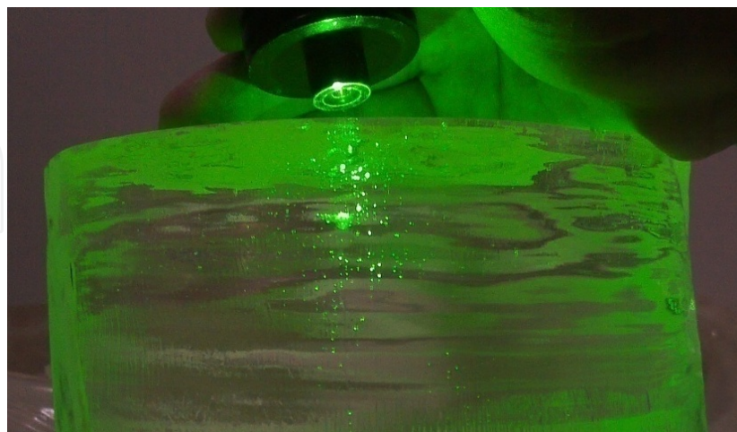
Figure 29. The bubble distribution of the sapphire boule grown by KY method.
