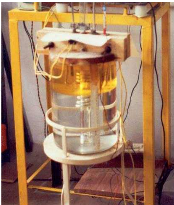
Figure 1. Transparent vertical Bridgman growth system.
