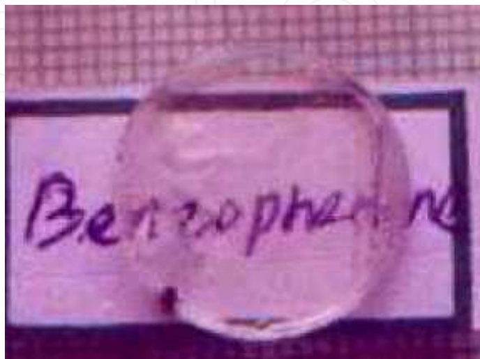
Figure 7. Prepared specimen from the \mu T-CZ grown crystal.
