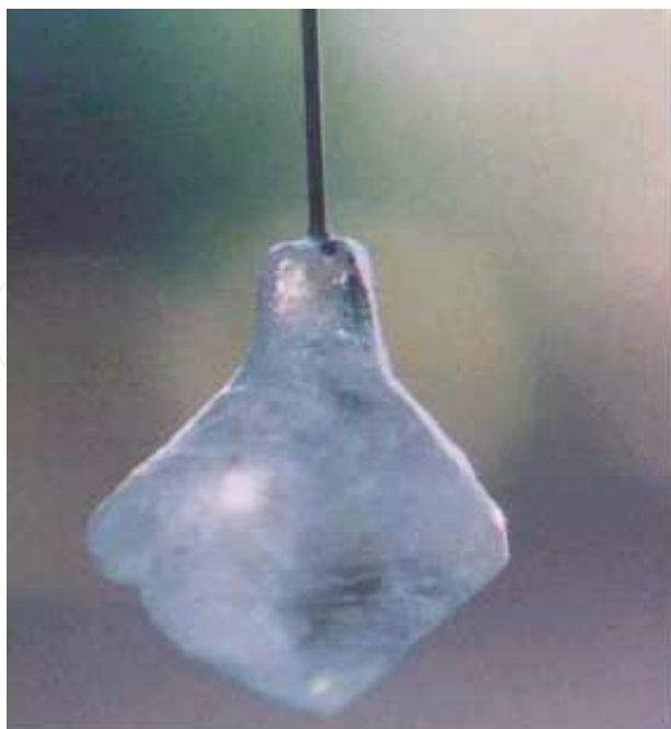
Figure 6. Grown crystal with high shoulder angle.
