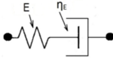
Figure 14 - Representation of the Maxwell model (adapted from [165])
