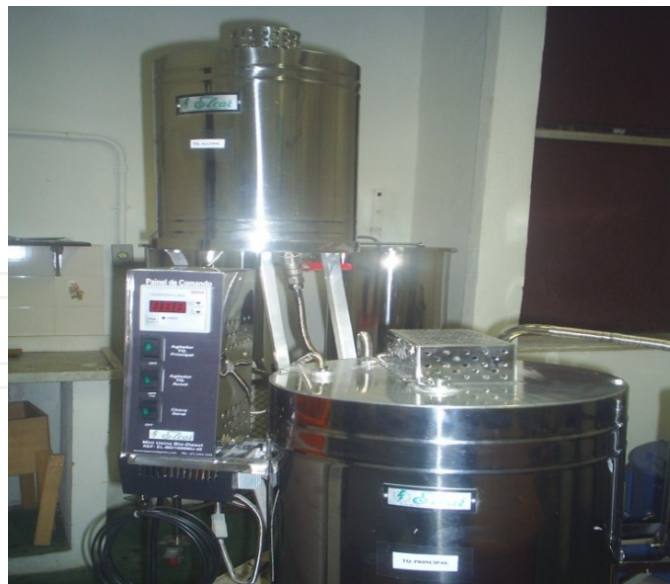
Figure 9. Small plant for the production of biodiesel
