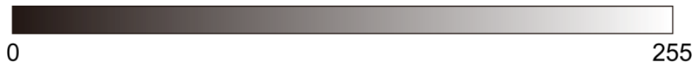
Figure 15. Illustration of the dynamic range of a gray scale image. Values between absolute black and white are divided into 255 levels. These levels are called “gray levels”.
