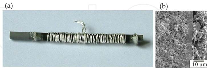
Figure 18. Prototype of a micro-tubular SOFC cell (a) and SEM topography of the cross-sectioned structure of NiO-YSZ-substrate, YSZ electrolyte and LSM cathode.
