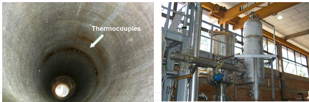
Figure 7. The internal thermocouples in the Measuring Station I, and the Thermal Stratification Experimental Facility (ITET) during assembly
