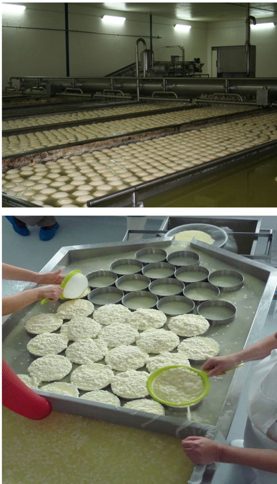
Figure 1. (Top) - Brine salting of cheeses in a large-scale plant processing 20 tons of cheese a day. (Bottom) - Small-scale unit processing 50 Kg per day of a traditional PDO cheese
