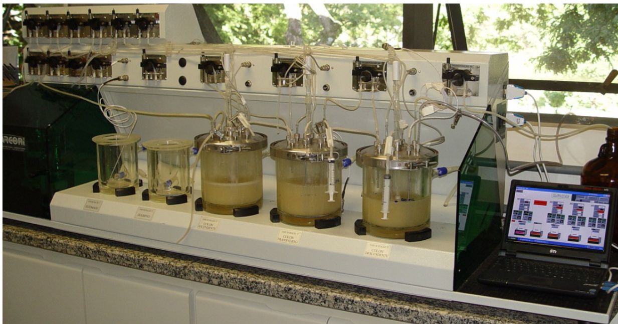
Figure 1. Computer controlled simulation of human microbial ecosystem (SHIME ®) housed in the Probiotics Research Laboratory of FCF/UNESP-Brazil. Sivieri et al.[53]
