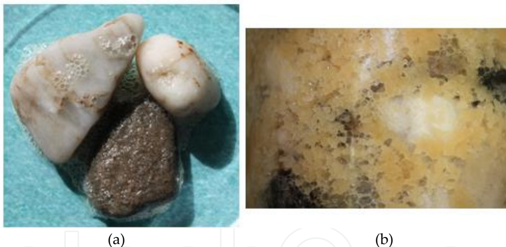
Figure 3. Images of the two structures formed by selected consortia of fermentative bacteria grown in a bioreactor on M9 medium containing molasses: (a) stones covered with bacterial biofilm (b) the granular sludge.
