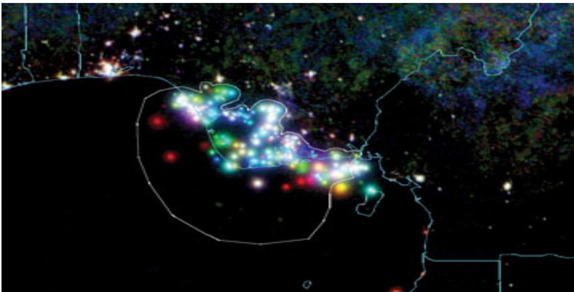
Figure 9. Satellite image shows Nigeria’s coastline burning bright with gas flares at night. The red dots represent gas flared in 2006, the green dots represent 2000 and the blue dots represent 1992. The white line encircles the flares associated with Nigeria.
