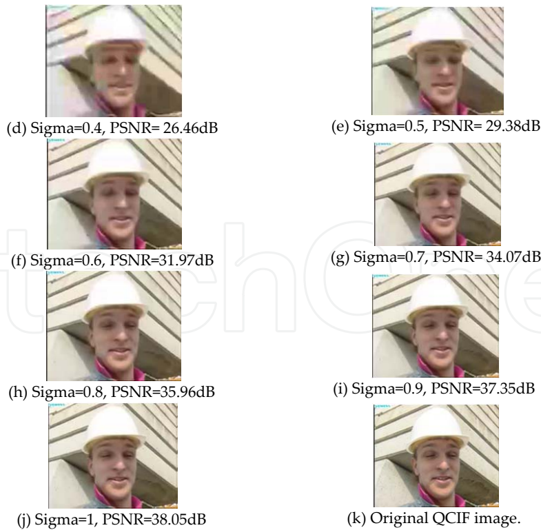
Figure 7. The 1 st frames of the QCIF “Foreman” sequence reconstructed by the central decoder corresponding to \sigma = 0.1 to 1.
