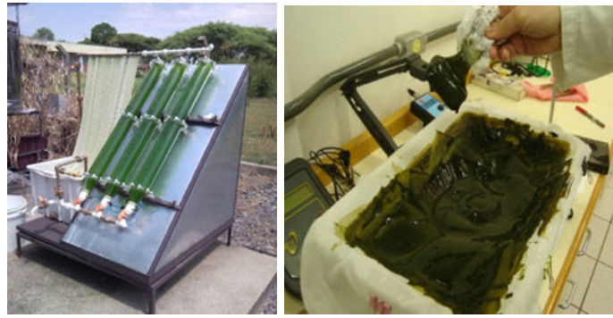
Figure 2. A) Mixed system prototype for microalgae production using a (1) scrubber, (2) tank, and (3) photobioreactor. B) Microalgae biomass in a mixed system separated by electroflotation [36].
