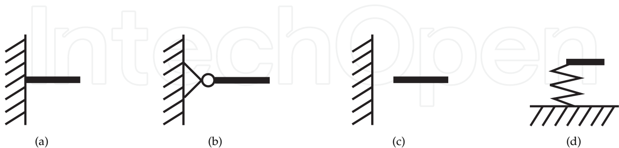
Figure 3. Schematics of four typical boundary conditions for deformable membrane mirrors showing (a) a clamped edge, (b) a simply supported edge, (c) a free edge, and (c) a spring supported edge type.
