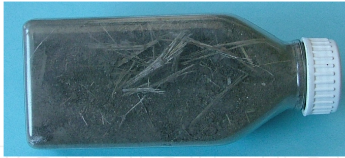
Figure 9. Tremolite asbestos fibres from the tailings dump of South African platinum mine. (Courtesy of Professor JI Phillips).
