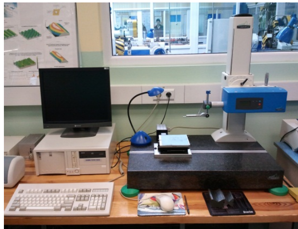
Figure 13. The view of stationary profilometer Hommelwerke T8000
