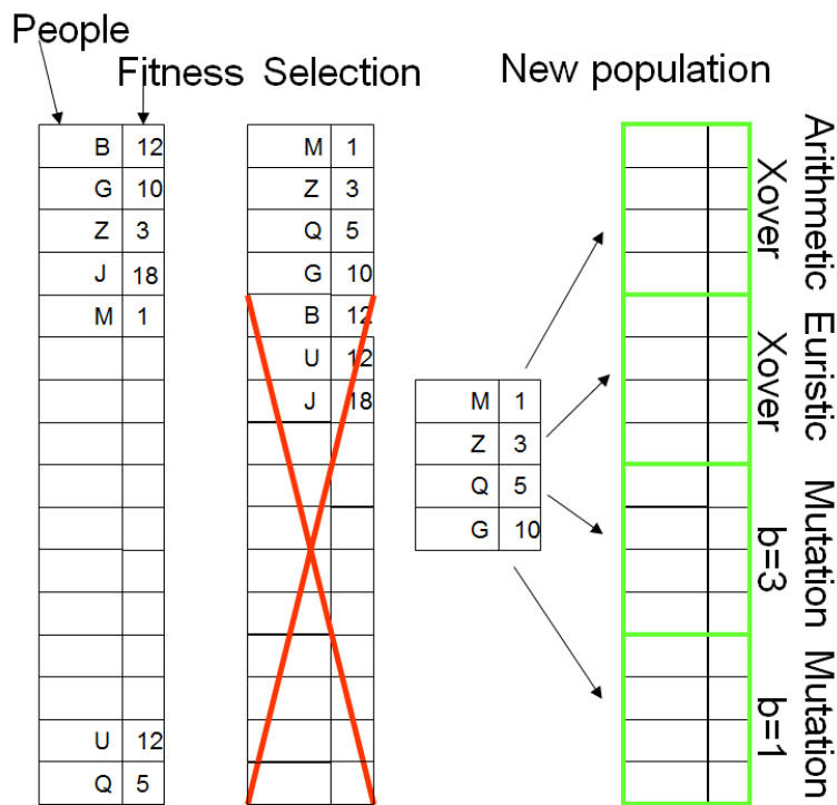
Figure 1. Diagram representing the genetic algorithm principle. The algorithm starts from a random population and then each individual is measured and the population is sorted according to its fitness. Then, some of the best individuals are selected for the generation of the next population.
