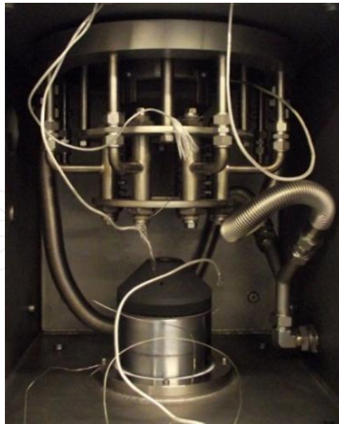
Figure 1. The image of the gas quenching system in the pulsed electric current sintering.
