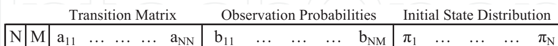
Figure 3. Chromosome array of the elements of an HMM, where N defines the number of states, and M the number of mixture components of the observation probabilities’ distributions.
