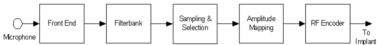
Figure 3. Audio signal path used in current filterbank strategies (Swanson, 2007).
