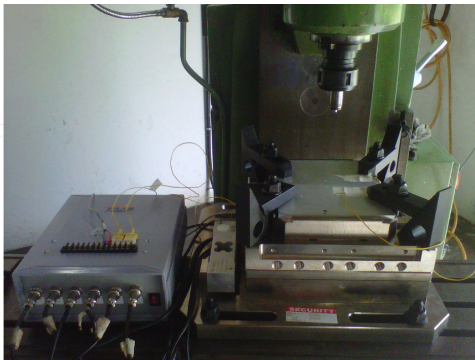
Figure 1. Friction stir welding experimental set up [5].
