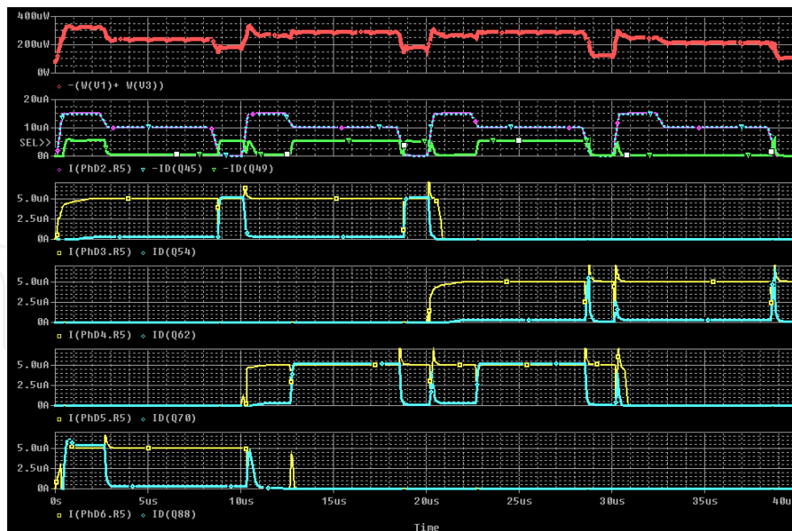
Figure 19. Diagrams of signals at modeling cell with an optical configuration for the desired function and the input photodiode
