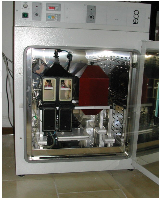
Figure 4. TEM cell placed vertically inside a cell culture incubator. TEM cell hosts, on both right and left side of the septum, two pyrex flasks over a 1.5 mm thickness plexiglas shelf.
