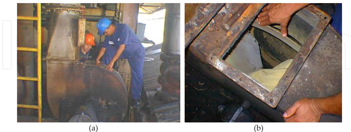
Figure 7. Photos of the attack-sites of samples: a) Ventilator extractor where samples were placed, b) Ventilator damp where samples were anchored.
