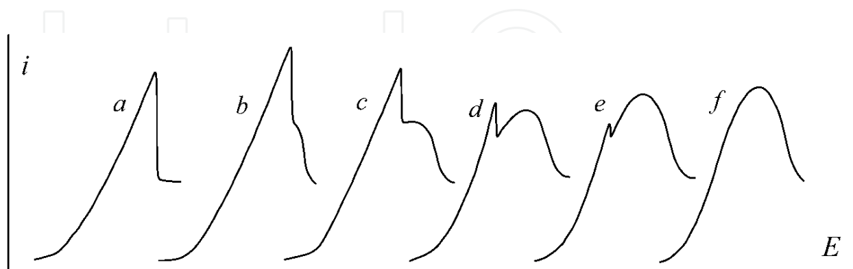
Figure 18. Another example of electrocatalysis of CPR type caused by adsorption of electroactive substance namely i.e. molecular oxygen. Solution 0.01 M KCl, exposed to air. The change of electrochemical response was caused by mercury head height lowering (processed literature data from Heyrovský, J.; Kůta, J. Principles of Polarography, Publishing House of the Czechoslovak Academy of Sciences: Prague 1965, Fig. XIX-23, p.457 [5]).
