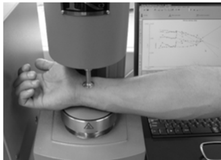
Figure 5. A rheometer can be used to determine the viscoelasticity of skin.
