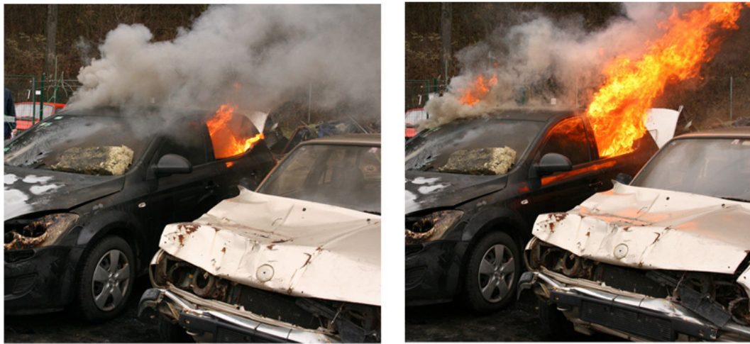
Figure 12. Full-scale fire experiment: passenger compartment fire
