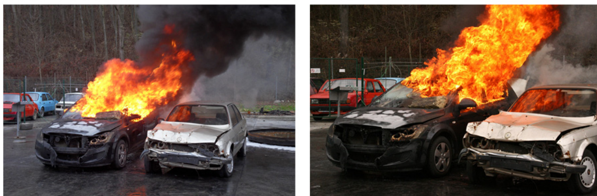
Figure 18. Full-scale fire experiment: spread of fire onto near-standing automobile
