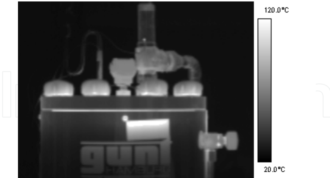
Figure 5. Marcet Boiler with logo that emits infrared radiation.
