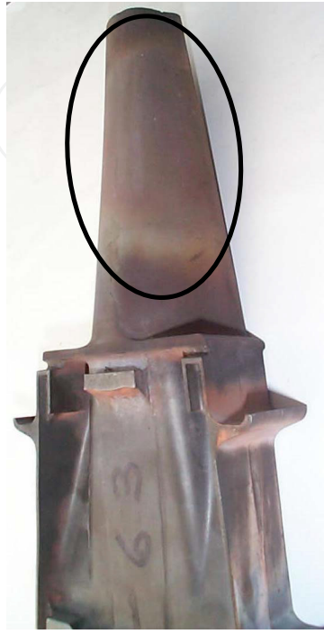
Figure 8. Oxidation (corrosion) marks on the blade [18].
