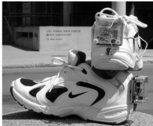
Figure 2. Piezoelectric-powered RFID shoes with mounted electronics.
