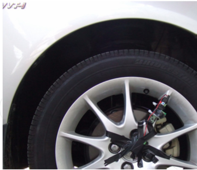
Figure 5. 3-axis accelerometer with the RF module mounted on the wheel.
