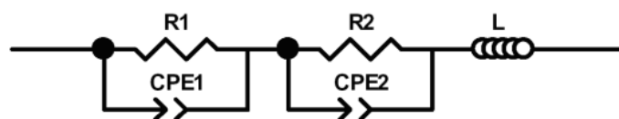
Figure 18. Equivalent circuit for SbSI@CNT gel prepared ultrasonically in methanol [13].
