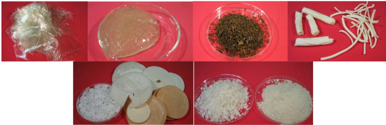
Figure 7. These are some ways you can shape the chitosan: films, gels, microspheres, tubes, sponges, powder
