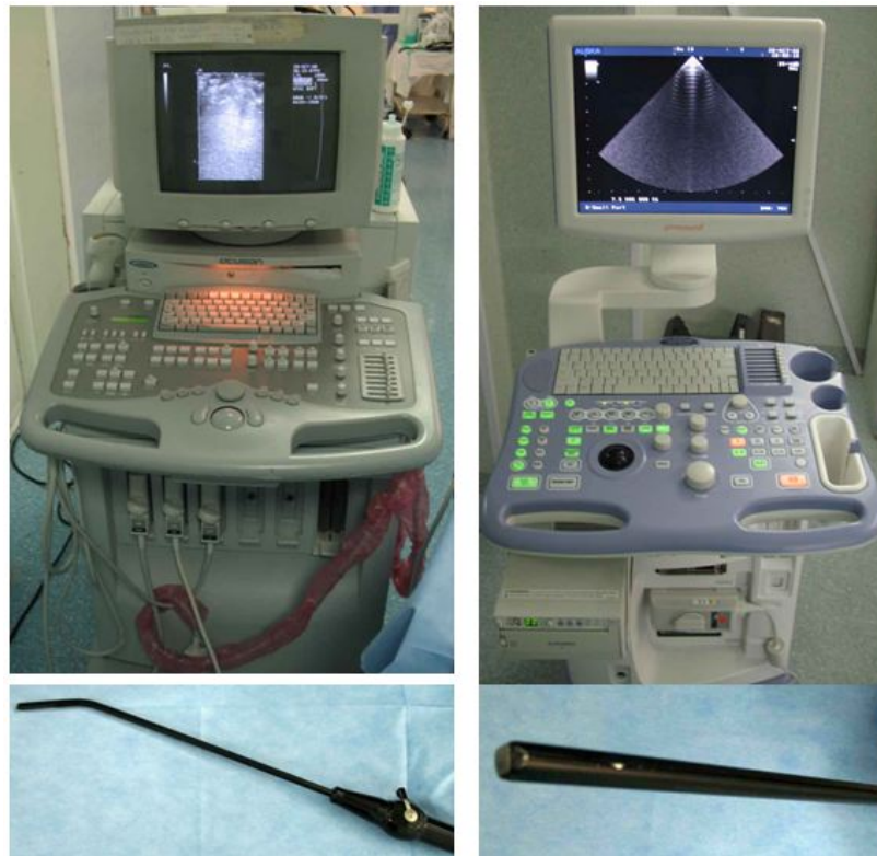
Figure 1. Ultrasound equipment. A. Ultrasound machine with flexible linear transducer for laparoscopy. B. Ultrasound machine with fixed convex transducer for laparoscopy
