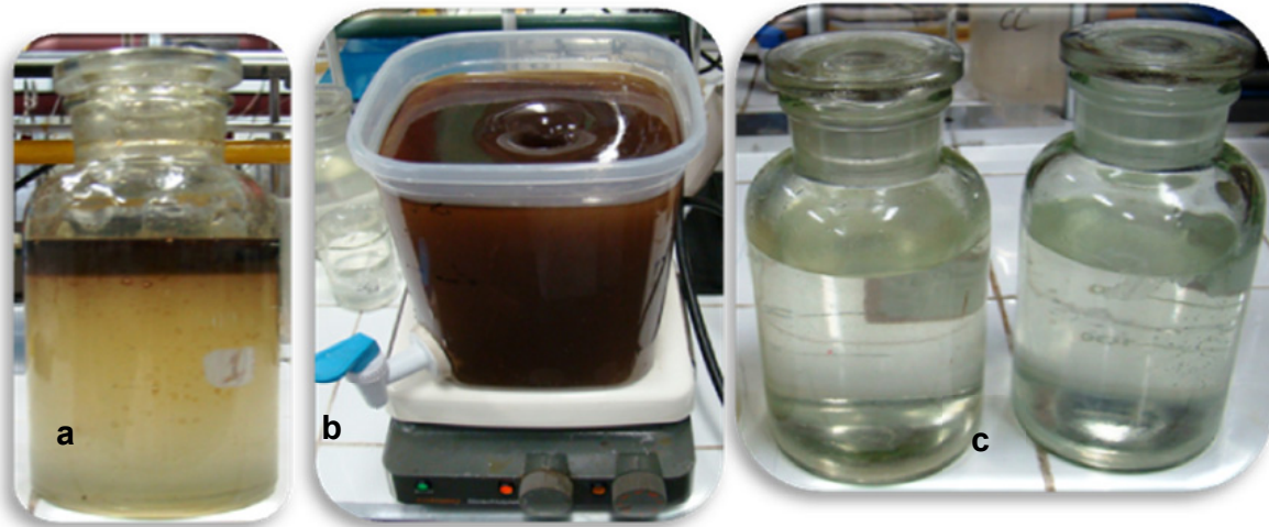
Figure 8. EF tests with high-salinity effluent. Legend: 60g / L NaCl: a) raw wastewater containing 60g / L of O&G; b) raw wastewater being mixed salt, for EF testing; c) effluent treated with AC (left) and DC (right) electroflocculation.
