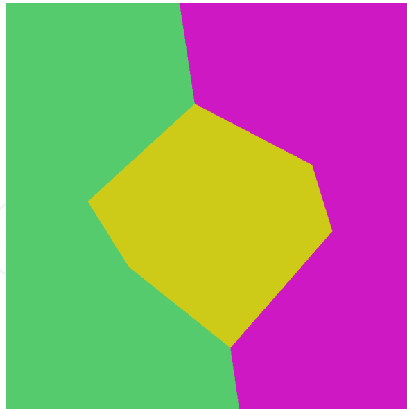
Figure 6. The computational domain is divided into three regions. The orientations of the solids in the central, left and right regions are \theta = 0^\circ and \phi = 0^\circ , \theta = 0^\circ and \phi = 60^\circ , and \theta = 0^\circ and \phi = 30^\circ , respectively.
