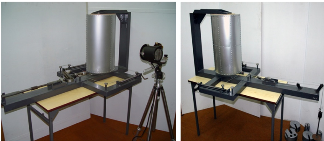
Figure 3. A stand for testing thin-shell structures subject to torsion: left – a version with a loading system controlling the displacement (turnbuckle), right – a version with a system controlling by force (gravitational).
