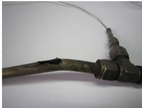
Figure 16. Damaged SUS coal powder feeding pipe occurred during the 8 bar and around 1,500°C gasification pilot plant test
