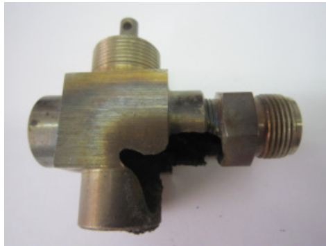
Figure 15. Damaged valve main body by the syngas explosion occurred during the 10 bar and around 1,500°C gasification pilot plant test
