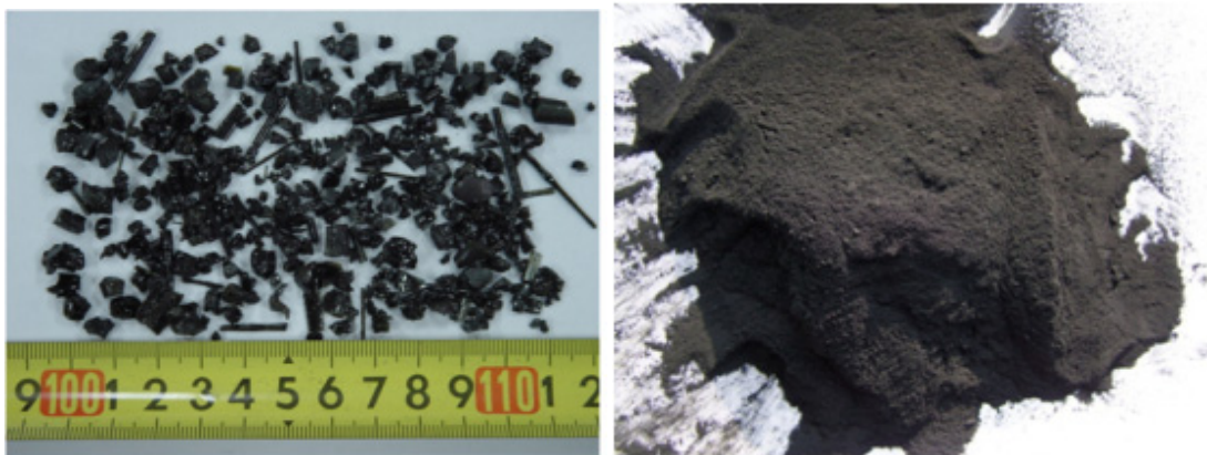
Figure 4. Slag(left) from slagging gasifier and fly-ash(right) from non-slugging gasifier
