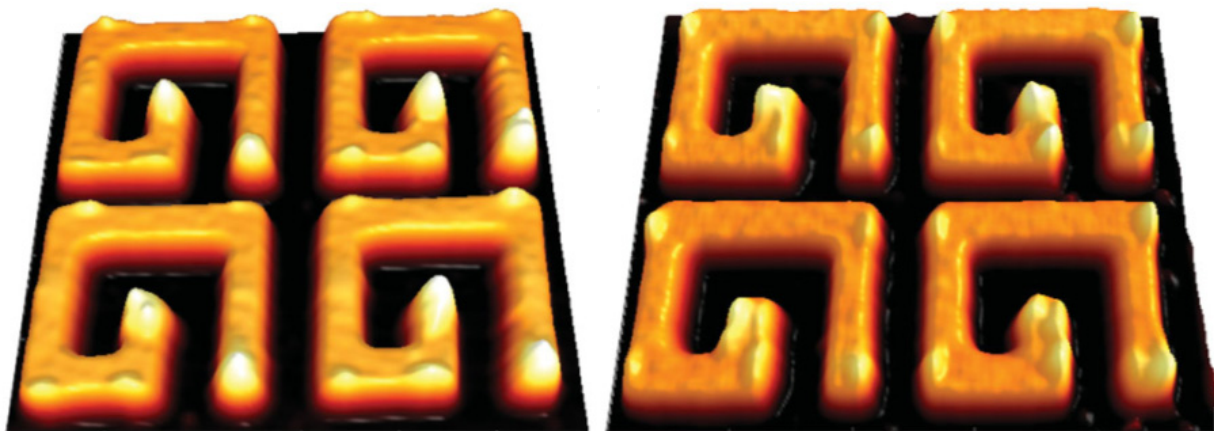
Figure 8. Illuminating the sample with femtosecond laser pulses produces a polarization dependent pattern of nanobumps with sharp tips on the sample surface [49]. Left: horizontally polarized light, right: vertically polarized light.
