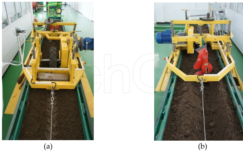
a – study of wheel – soil interaction; b –study of plough body – soil interaction.
