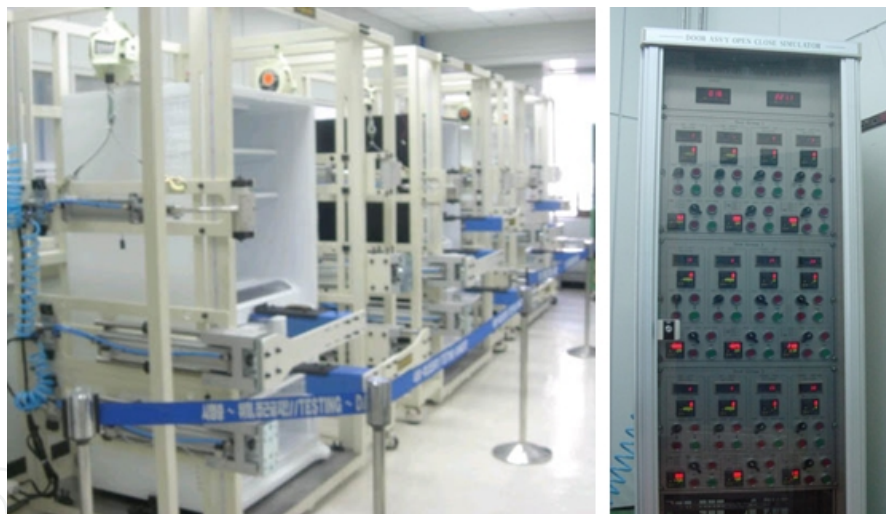
(a) ALT equipment and controller
